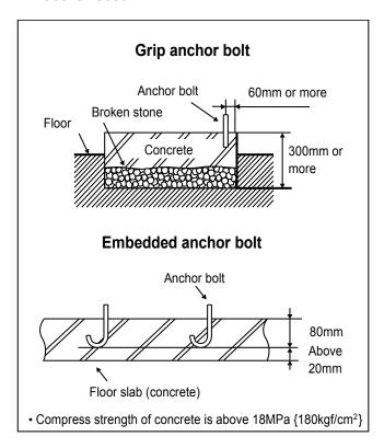
Illustration of grip type and embedded type anchor bolt
