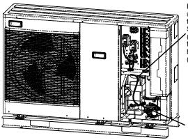
How to guide cable / cord to bushing
