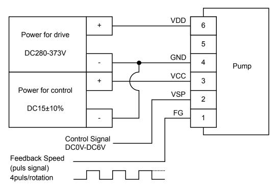
Control signal is analog voltage (DC0V-6V) generated by microcomputer PWM port. Microcomputer can change analog voltage by changing PWM duty.
