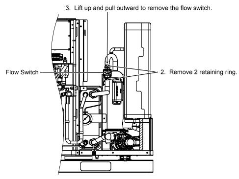
1. Disconnect the connector of CN-FLOW from the Electronic Controller Board.
