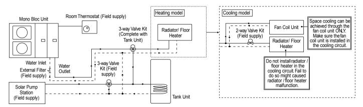
Diagram 3.1: Typical Water Piping Installation
