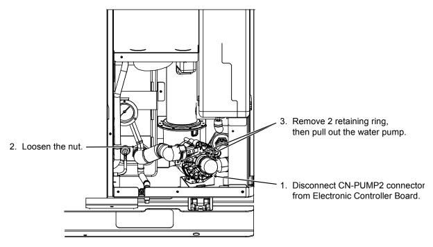
⚠ When reinstall the water pipe, use grease or water at the joining.
